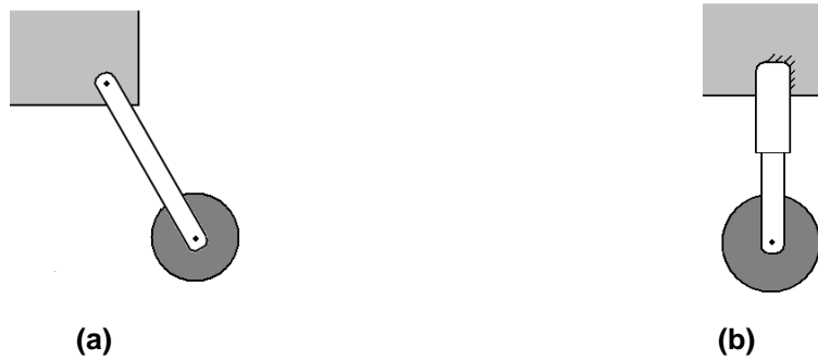
Figure 1.3 (a) 1 motion DOF articulation using revolute joint and (b) 1 motion DOF articulation using prismatic joint.
